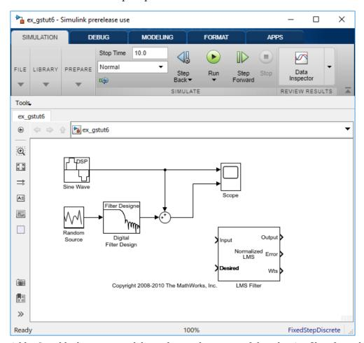
Add a Sum block to your model to subtract the output of the adaptive filter from the sinusoidal signal with low frequency noise. From the Simulink Math Operations library, drag a Sum block
