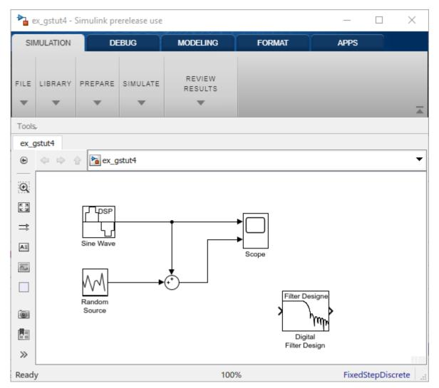
Incorporate the Digital Filter Design block into your block diagram by placing it between the Random Source block and the Sum block.
